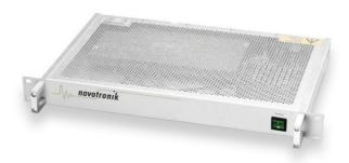
The two channel antenna multicoupler is used for compact distribution of two independent RF and VHF/UHF signals. Each channel provides 4 decoupled outputs. The frequency ranges covers 1.5...30 MHz (channel 1) and 20 ... 3000 MHz (channel 2).
