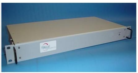
Terrasat's Indoor IBUC Power Supply, model PSUI-1248, runs on AC mains power and provides DC power to the IBUC through a multi-conductor 16 AWG cable. The units are packaged in rack-mountable chassis with internal cooling fans.
