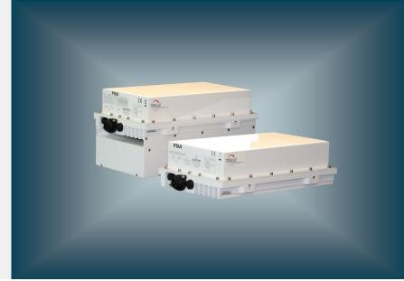
Terrasat's Outdoor BUC Power Supplies run on AC mains power and provide 48 VDC nominal power to the IBUC through a multi-conductor 16 AWG cable.
